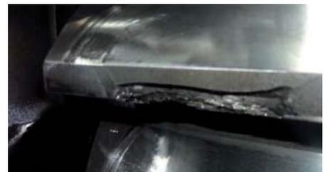
*Tooth gear failure on Banbury mixer gears due to overloading*
