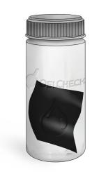
Send the filter fleece in a brand new plastic bag or clean bottle, e.g. from an analysis kit, to OELCHECK. Enclose the completed Sample Information Form or complete it online.
