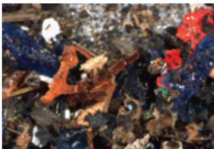
Impurity extracted on the test membrane
