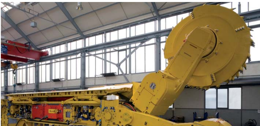
An Eickhoff SL 1000 shearer loader undergoing final assembly at the factory in Bochum.
