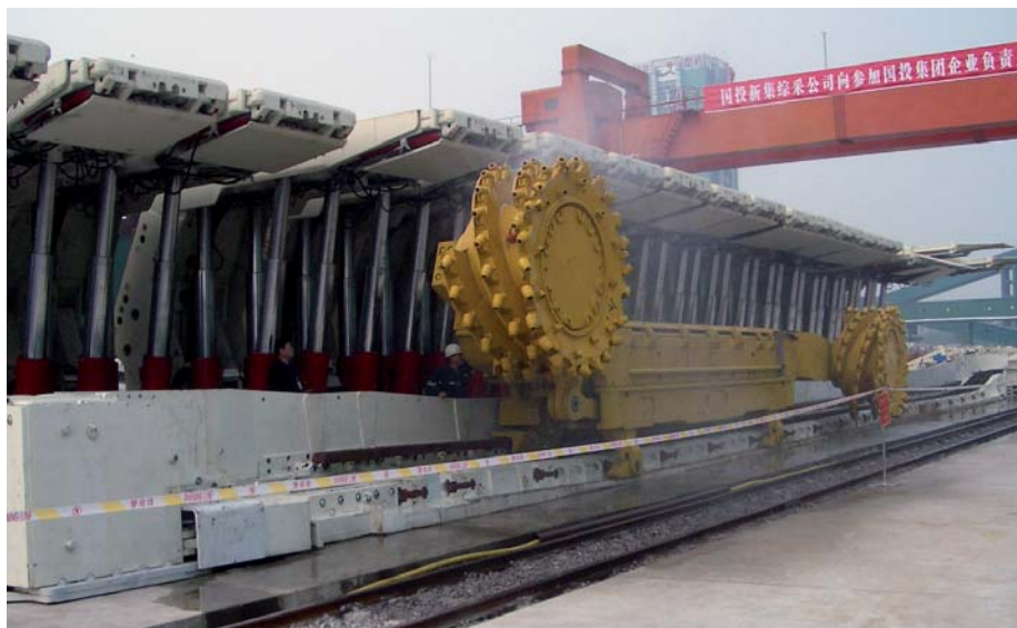
Assembly of an Eickhoff shearer loader prior to use in underground mining in Huainan/China.
