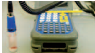
RULER with grease specimen
