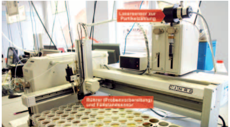
The innovative particle counter in the OELCHECK laboratory already offers clear-cut advantages.
