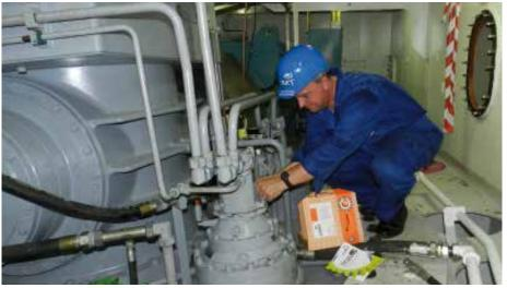
Removal of a representative oil specimen from the engine of a marine engine.
