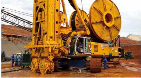
Bauer trench cutters allow trench walls to be constructed even in difficult ground conditions and extreme climatic conditions.
