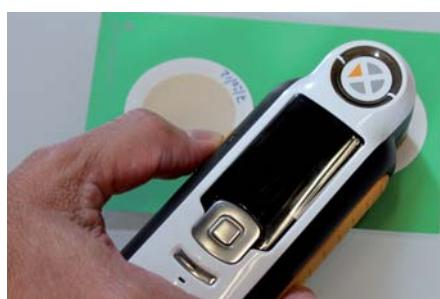
MPC-Test (Membrane Patch Colorimetry)
