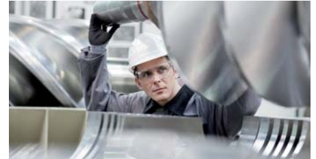
Inserting a rotor into the plain bearing
