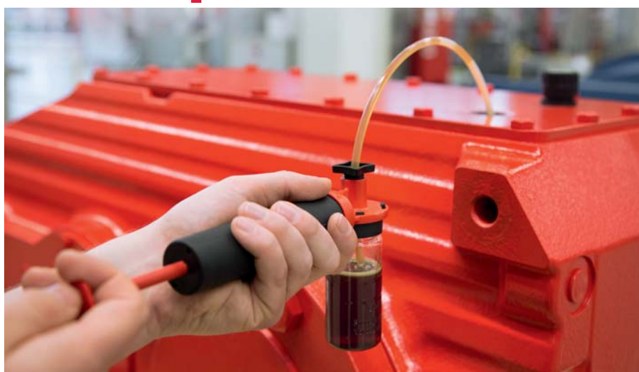
Sample from an SEW-EURODRIVE large gear. OELCHECK oil analyses are the perfect complement to SEW-EURODRIVE's Condition Monitoring Service.
