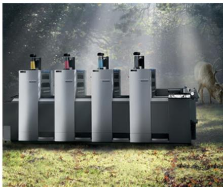
A CLP 150-type mineral oil-based industrial gear oil is usually used to lubricate printing presses. Depending on the type of press and number of print works, between 50 and 150 litres of gear oil are required.
