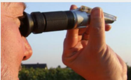
A typical application is measuring the sugar content of grape must, which is a criterion in determining the quality of wine. Particularly in the case of foodstuffs, the refractive index is still traditionally given in °Brix, or in the case of wine in °Oechsle.
