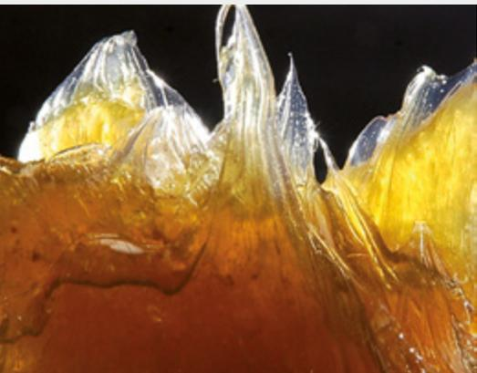
Lubricating greases are commonly used in situations where a lubricating surface cannot be perfectly supplied with oil. In addition to providing optimal lubrication, in many cases lubricating greases must also seal lubricating surfaces and protect moving parts against wear and contamination. They should attenuate shock loads, and ideally they should be
