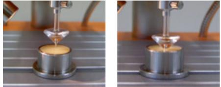
Cone penetration - cone above grease and after 5 minutes
