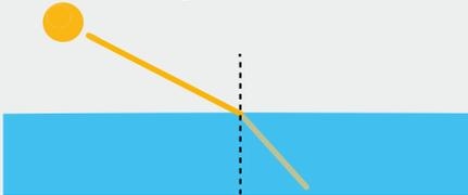
The refractive index has its origins in optics. When light passes from one medium into another, the rays of light are refracted at the junction, changing their direction and their speed. Figuratively speaking, the ray of light bends. The strength of the effect depends on the refractive index of the medium.
