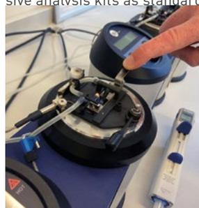
Ignition test in a Setaflash flashpoint tester
