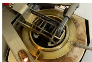
Determination using the Cleveland method with an open crucible
