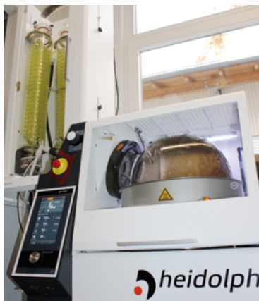
Heidolph Hei-Vap rotary evaporator (with Hei-Volume Distimatic Pro automation) for heptane recovery
