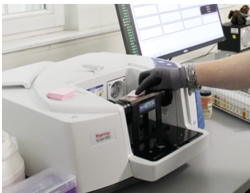
Thermo Scientific Nicolet APEX IR with HATR cell for IR spectroscopy of lubricating greases
