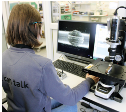
Keyence VHX-S660E microscope for measuring the wear marks of Brugger and VKA test
