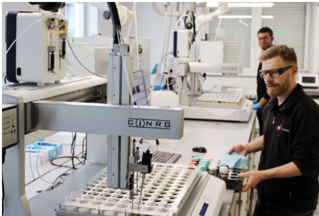
Two additional CINRG APC3 particle counters for determining particle numbers and sizes as well as purity class according to ISO 4406
